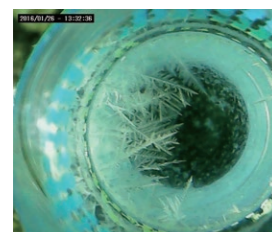
A top view of ice dendrite crystalized in horizontal magnetic field of 10 T with gradient. Trunk of dendrite extended on one side of a reactor was extended along magnetic flux.
